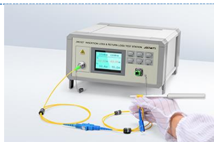
Return Loss Testing
