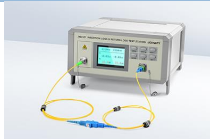
Insertion Loss Testing
